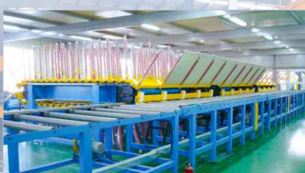
PANEL COOLING MACHINE
