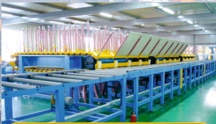
PANEL COOLING MACHINE
