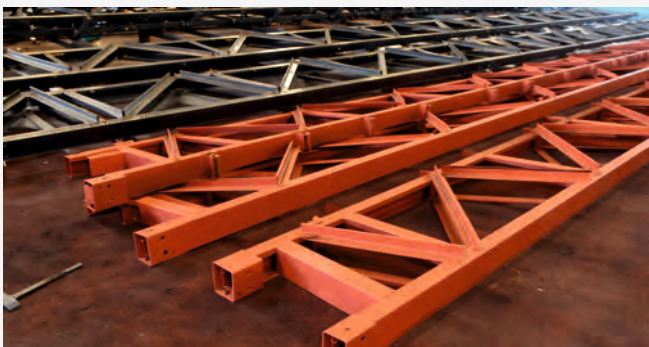
UN-PAINTED FLOOR JOIST
