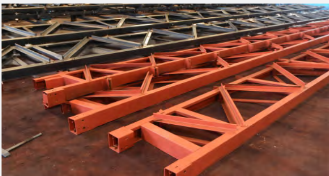
UN-PAINTED FLOOR JOIST
