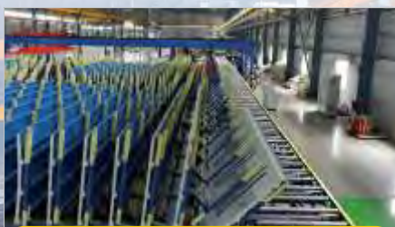
PANEL COOLING MACHINE
